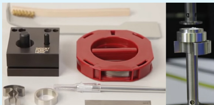
Figure 3. TA Instruments ARES-G2 melt ring kit, allowing for sample loading from pellet feedstock.
