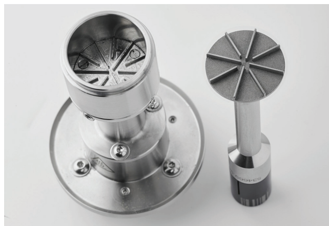
Figure 1. Shear cell with serrated upper plate and cup to prevent powder slip.
