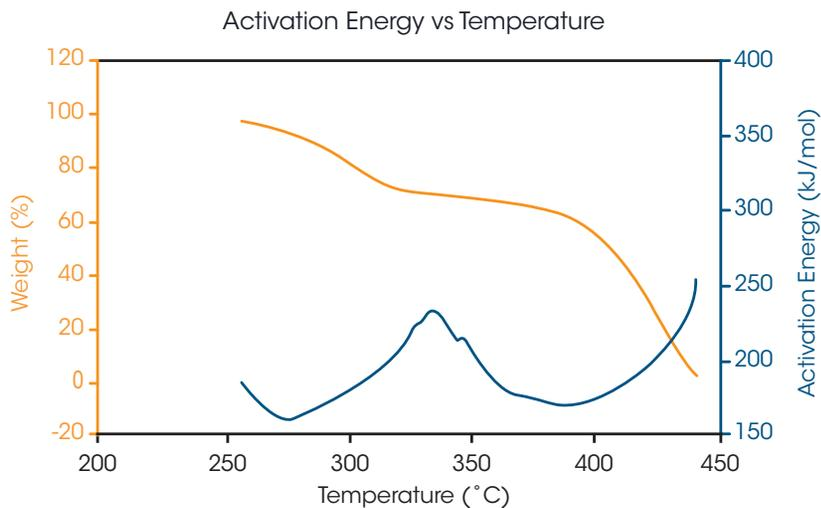
TA's patented MTGA\* is another TA Instruments innovation that offers advantages for material decomposition studies. Developed from the proprietary heater control technology utilized by Hi-Res TGA and MDSC, MTGA produces model-free kinetic data. Activation energy can be calculated real-time and studied as a function of time, temperature, and conversion.
