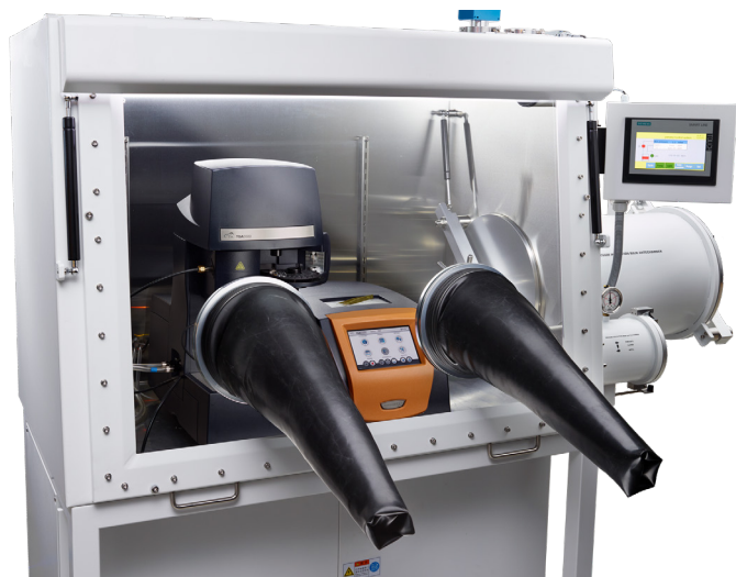
Figure 1. Discovery TGA 5500 installed in a glovebox
