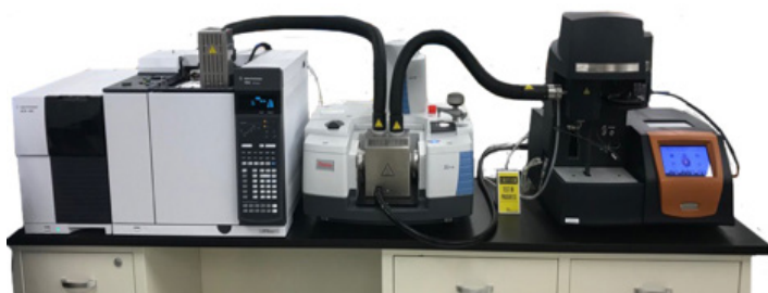
Figure 2. TGA, FTIR, and GC/MS Connected Using Redshift Interface
