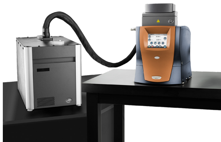
Figure 1. TA Instruments Dynamic Mechanical Analyzer with humidity control accessory
