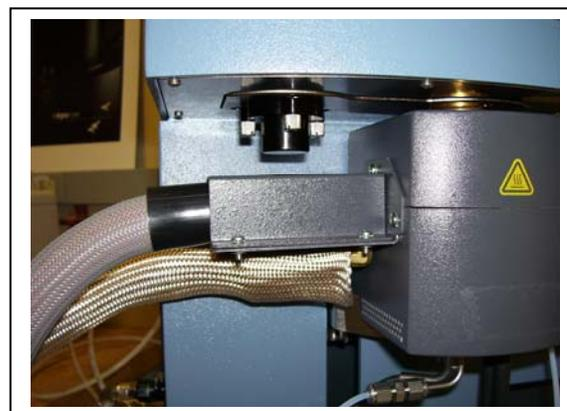
**Figure 2. Interface with MS/FTIR attached**
